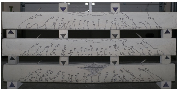
Fig. 13. Marked cracks on the S7, S8, and S9 beams (from the top)
