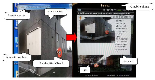
Fig. 4. Image-recognition-based mechanism for a Class A fire
