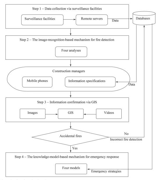
Fig. 2. Information flow from fire detection to emergency response
