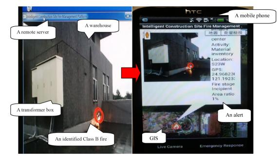
Fig. 5. Image-recognition-based mechanism for a Class B fire
