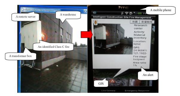
Fig. 6. Image-recognition-based mechanism for a Class C fire
