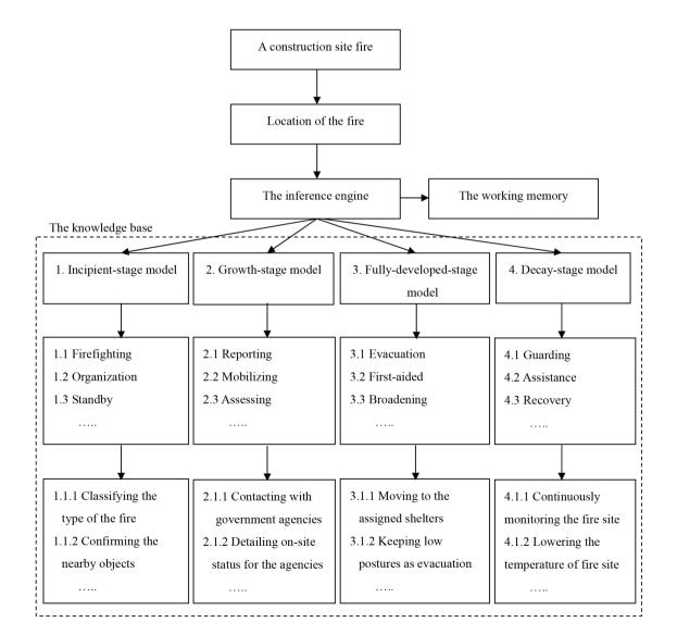
Fig. 3. Framework of knowledge-model-based mechanism
