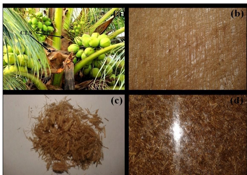
Figure 1. (a) Coconut palm, arrows show woven leaf sheath, (b) naturally woven coconut leaf sheath, (c) chopped coconut leaf sheath; and (d) chopped coconut leaf sheath-reinforced PP composite.
