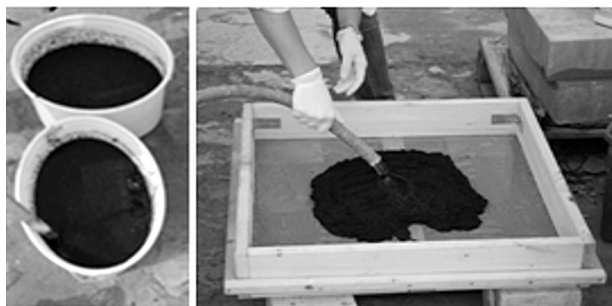
Fig. 5. Pre-treatment of rubber particles in the saturated calcium hydroxide solution
