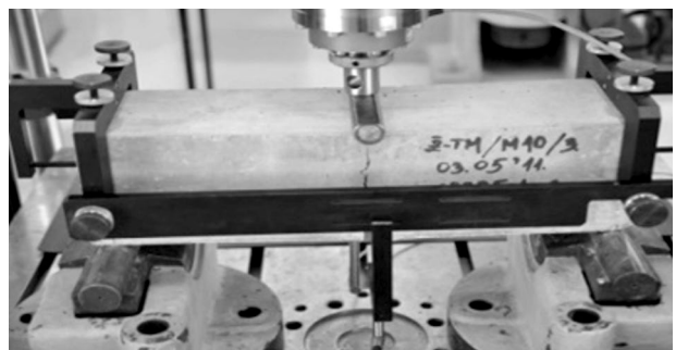
Fig. 6. Test setup for the three point bending test
