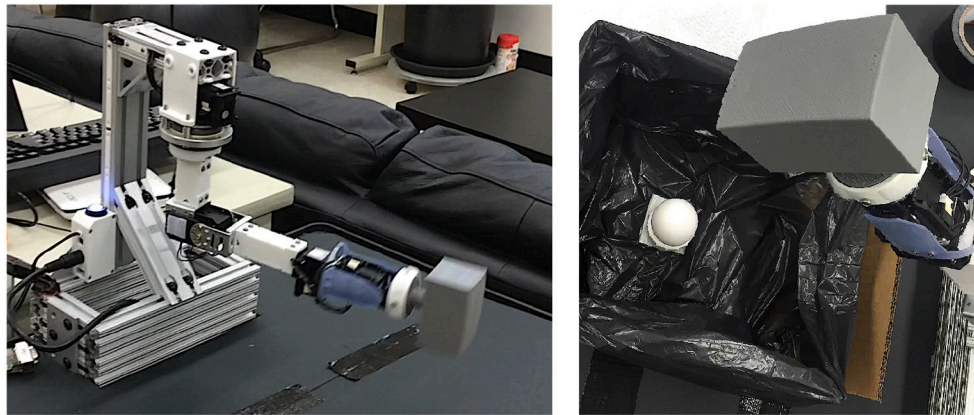
FIGURE 4 | Experimental setup, showing the robot arm in motion for the first experiment (Left) and the robot arm poised to impact an egg during the second experiment (Right).
