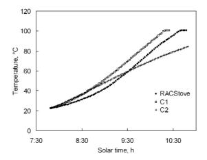
Figure 9: Performance for  $\theta$  = 21°, with tracking and averaged irradiance G<sub>DN</sub> = 896 W/m<sup>2</sup> (Brooks, 2006)
