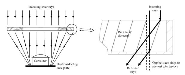
Figure 1: Schematic of RACStove operation for a horizont ally-aligned ring array with concentrated sunlight focused on oven base plate (left), and detail of reflected solar ray path between mirror elements (right)
