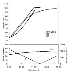
Figure 11: Performance for the stationery test (ovens facing true north), with lower graph indicating beam irradiance and solar angle of incidence for the prototype RACStove (Brooks, 2006)
