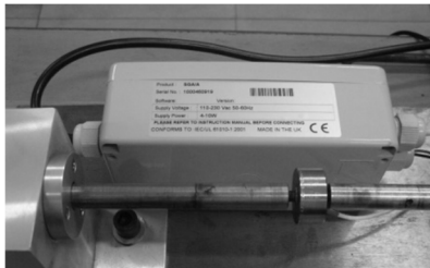
Fig. 9. Thrust force sensor and modulator
