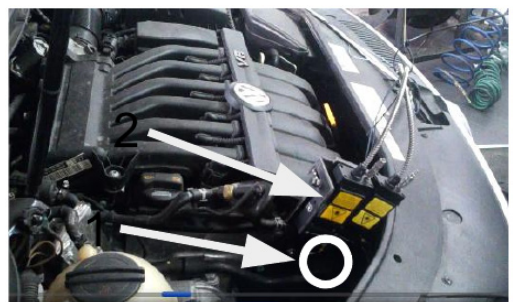
Fig. 7. Engine chamber and used sensors. 1 – three-axis accelerometer, 2 – heads of laser vibrometers
