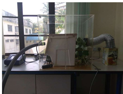
Fig. 2. Photograph depicting experimental testing apparatus used to expose the modular botanical air biofilter to a single pulse event of particular matter.
