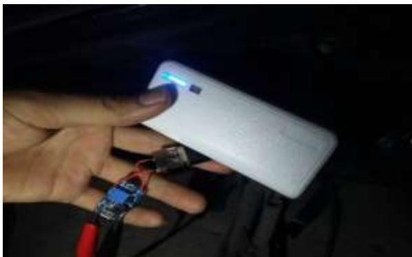
Gambar 14 Pengisian arus di power bank
