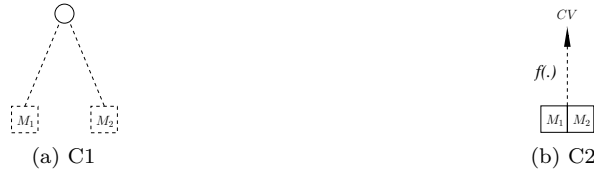
Figure 1: A (2-ary) node using convention C1 (left) or C2 (right), drawn as a solid bold line. At the left, a node is an image by f and is represented with a circle. At the right, it consists of an entire input to f , e.g. the message blocks M_1 and M_2 (the coding bits are neglected). The result of f is either the final digest or a chaining value ( CV ) which takes place in another input to f .
