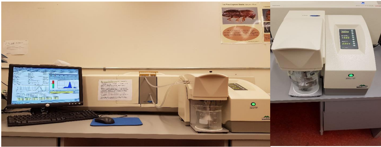
Figure 16: Malvern Mastersizer Hydro 2000S to measure the droplet size of the particle
