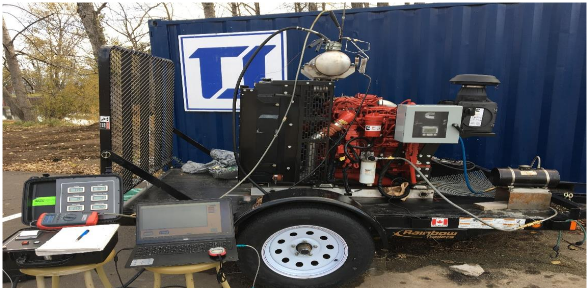
Figure 21: Cummins Engine Testing Setup
