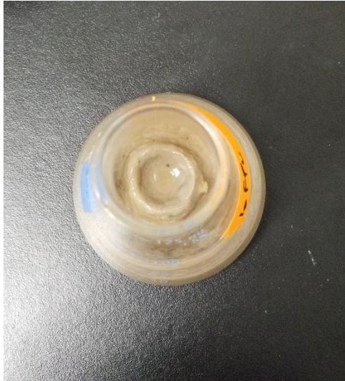
Figure 4.7: Irregular mixing pattern caused due to high solid loading.
