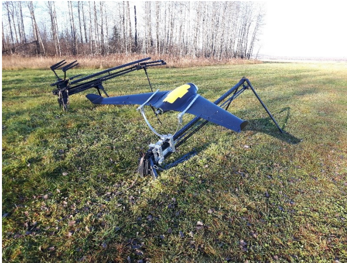
Figure 18: Skywalker X8 Sitting on Launch Catapult
