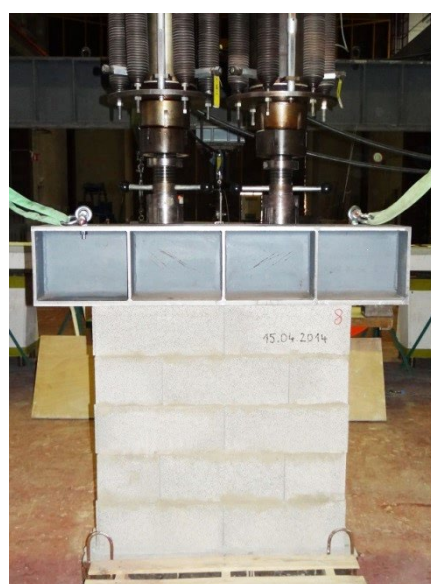
Fig. 5. Collar jointed wallettes ready for testing
