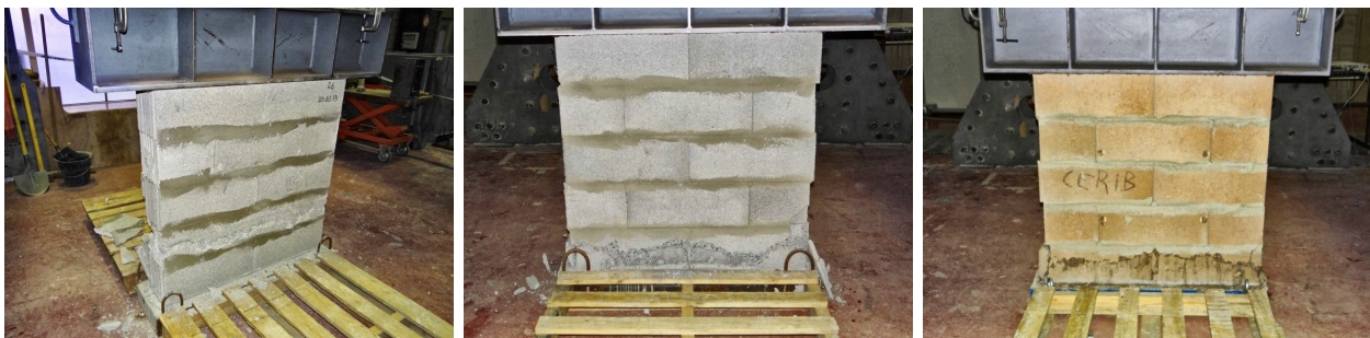
Fig. 7. Typical failure of lightweight aggregates masonry wallettes
