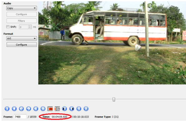
Fig. 4. A view of extraction of entry and exit time of vehicles using Avidemux 2.5
