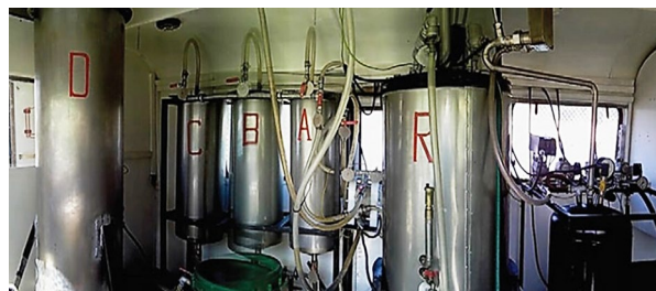
Fig. 2. A panoramic view of a mobile diesel production plant, built on a chassis of a Star 266 vehicle – the transesterification reactor (R) with the post-reaction mixture separators (A, B, C) (Piętak et al. 2012)
