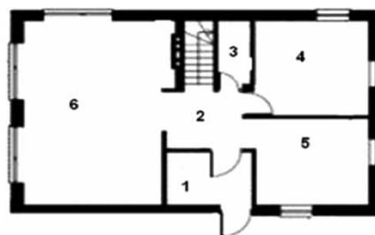
Fig. 5. The plan of the ground floor of the investigated house: 1 – anteroom; 2 – hall; 3 – toilet; 4 – kitchen; 5 – office room; 6 – living-room
