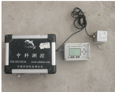
a) The blasting vibration monitoring system b) The layout of blasting vibration monitoring points Fig. 3. The blasting vibration monitoring system and layout of blasting vibration monitoring points
