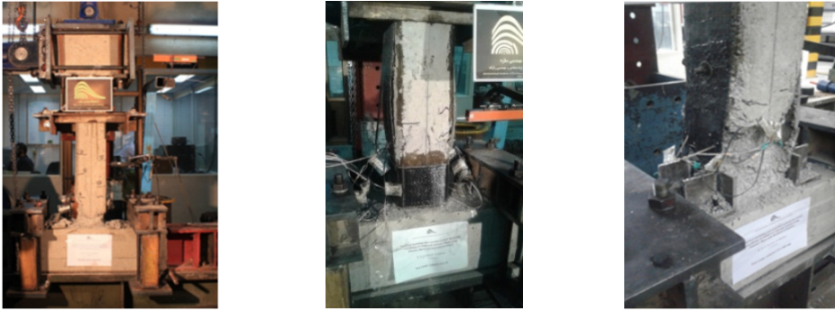
Fig. 5. Failure mode of C0, C1 and C2
