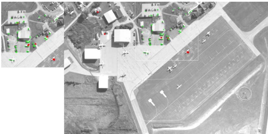
Fig. 8. Feature detection with ORB algorithm. Feature matching of two images
