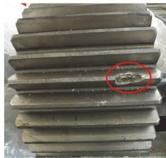
Fig. 19. The damaged planetary gear
