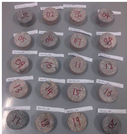
Fig. 8. Rock samples before SHPB impact test
