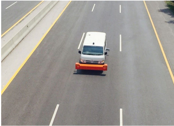
Fig. 3. Pavement roughness data collection using instrumented vehicle
