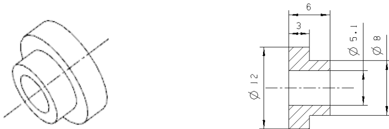
Fig. 5. Structure of rubber shock absorber
