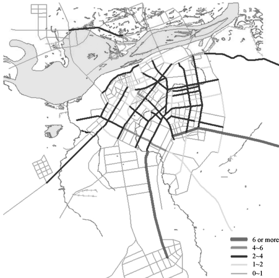
Fig. 1. The prototype of traffic volume intensity united 10,000 pcu on road segment networks in Harbin
