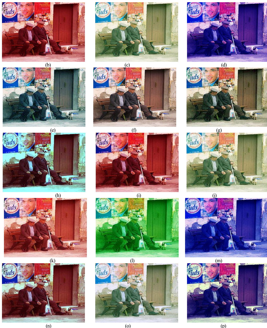
Fig. 3. Two-men image (a) Reference, (b) Red cast (c) Green cast, (d) Blue cast, (e) proposed corrected Red cast (f) proposed corrected Green cast (g) proposed corrected Blue cast (h) Grey world corrected Red cast (i) Grey world corrected Green cast (j) Grey world corrected Blue cast (k) max-RGB corrected Red cast (l) max-RGB corrected Green cast Two-men image (m) max-RGB corrected Blue cast, (n) shades of grey corrected Red cast, (o) shades of grey approach corrected Green cast (p) shades of grey approach corrected Blue cast
