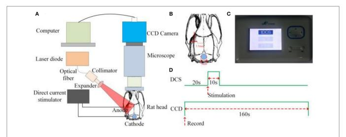
FIGURE 1 | Experimental setup for LSCI and DCS (A) Schematic of the experimental setup. (B) AP and ML coordinates of position, 3.5 and 2.5 mm, respectively, of the anode-stimulating electrode. (C) Photograph of the direct-current stimulator. (D) Sequential diagram of the experiment.
