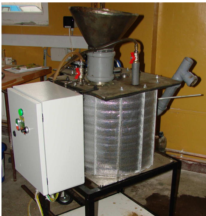
Fig. 1. The experimental anaerobic vertical digester
