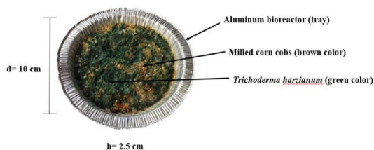
Fig. 1: SSF system in aluminum tray at 96 h employing corn cobs, a sole carbon source, for the microorganism's growth and xylanase production.
