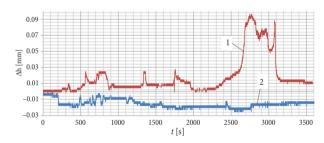
Fig. 11. Curves of variation of specimen width in the medium of liquid nitrogen (explanations are given in the text)
