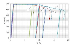
Fig. 8. Stress–strain curves for titanium alloy VT22: 1 – ST; 2 – ST + DNP ( $F_{imp} = 60 \text{ kN}$ ) + ST; 3 – HLN + ST; 4 – DNP ( $F_{imp} = 60 \text{ kN}$ ) before the yield point of the alloy HLN + ST
