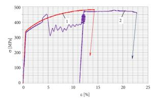
Fig. 3. Stress–strain curves of aluminum alloy D16: 1 - ST; 2 - ST + DNP ( $F_{imp} = 89.6 \text{ kN}$ ) + ST
