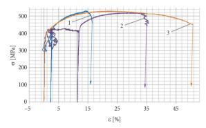
Fig. 6. Stress–strain curve for stainless steel 04Kh18N10: 1 – DNP ( $F_{imp}$  =68.5 kN) + ST; 2 – HLN + DNP ( $F_{imp}$  =59.9 kN) + ST; 3 – ST in the initial condition at t = 20°C
