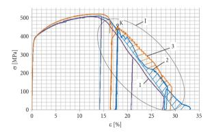
Fig. 7. Curves of macrocrack growth in specimens from stainless steel 04Kh18N10 with openings: 1 - ST, 2 - ST + DNP ( $F_{imp} = 7.4$  kN); 3 - ST + DNP ( $F_{imp} = 12.7$  kN) with the application of colloid solution
