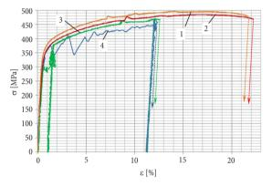
Fig. 4. Stress–strain curve of aluminum alloy 2024-T3: 1 – ST at 20°C; 2 – HLN, warming up to 20°C + ST; 3 – ST + DNP ( $F_{imp}$  =90.4 kN), HLN, warming up to 20°C + ST; 4 – ST + DNP ( $F_{imp}$  =111.8 kN), HLN, warming up to 20°C + ST
