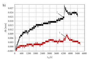
Fig. 10. Width measurement of specimens from the alloy 2024-T3 during HLN for 1 hour: a – specimen in a bath with liquid nitrogen; b – data on the specimen width variation (1 – initial condition; 2 – after the DNP implementation)
