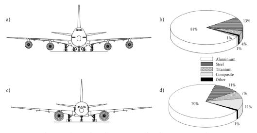
Fig. 1. Combination of materials used in Boeing aircrafts: a, b – Boeing-747; c, d – Boeing-777 (Dursun, Soutis 2014; Jones *et al.* 2005)
