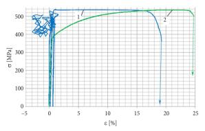
Fig. 5. Stress–strain curves for stainless steel 04Kh18N10: 1 – ST + DNP ( $F_{imp}$  = 103.9 kN) + HLN + DNP ( $F_{imp}$  = 109.3 kN) + HLN + ST; 2 – ST
