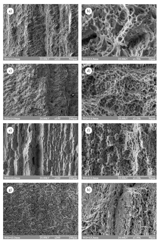
Fig. 12. Scanning Electron Microscope (SEM) images of fracture of alloy VT22 after: a, b – ST; c, d – ST + DNP ( $F_{imp} = 60 \text{ kN}$ ) + ST; e, f – HLN + ST; g, h – DNP ( $F_{imp} = 60 \text{ kN}$ ) before the yield point of the alloy + HLN + ST
