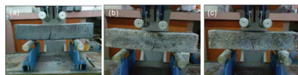
Fig. 6. Flexural failure of S1/50 (a); S2/50 (b); and S3/50 (c)
