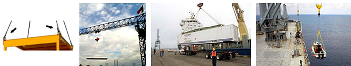
Fig. 1. Sling wire rope application in lifting and transport processes
