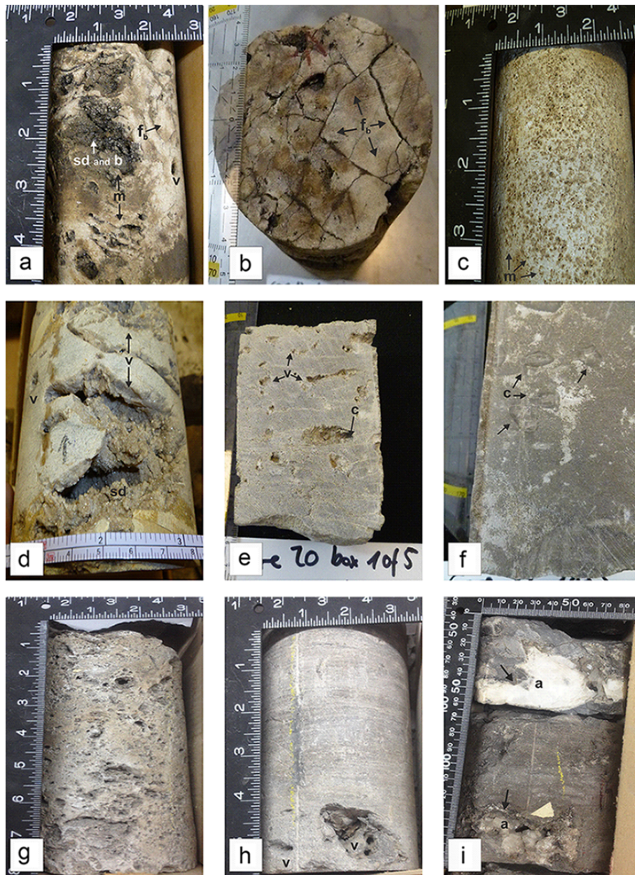
Plate A1. Representative core samples of the Leduc Formation from the RMRT and the SCCC. Except for (f), all samples are dolostones. The scale bar is in inches and centimetres. (a, b) Light grey stromatoporoid floatstone (medium crystalline) with large vugs and abundant subvertical fractures ( f_b ) filled with bitumen (1843.1 m b.g.l., 5-22-48-27W4, RMRT). The notation “sd and b” stands for saddle dolomite covered with bitumen. (c) Light grey Amphipora grainstone with small-sized tubular molds (1957 m b.g.l., 5-22-48-27W4); “m” indicates molds. (d) Coarse-crystalline stromatoporoid floatstone–rudstone with large vugs that are lined with saddle dolomite (sd: saddle dolomite, 1993.4 m b.g.l., 5-22-48-27W4). (e) Core slab of skeletal wackestone–floatstone with calcite cement (“c”) crystals lining scattered molds and vugs (4290 m b.g.l., 10-31-37-9W5, RMRT). (f) Core slab of nonporous, nondolomitized mudstone facies in the Strachan pool close to the Rocky Mountains (4306.8 m b.g.l., 10-31-37-9W5). Brachiopod molds (black arrows) are filled with microsparitic calcite cement (“c”). (g) Coarse-crystalline packstone–floatstone facies with a variety of molds of corals and stromatoporoids (4095 m b.g.l., 2-36-54-23W5M, SCCC). (h) Fine-crystalline dolomudstone with scattered large vugs (4159.75 m b.g.l., 2-36-54-23W5M). (i) Irregularly shaped masses of replacive anhydrite (“a”) in medium to dark grey replacement dolomite. The anhydrite near the bottom of this photo is partially infiltrated by “dead oil” (4164.78 m b.g.l., 2-36-54-23W5M).
