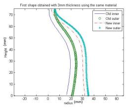
Figure (9): First obtained shape of the candle holder after changing the volume.
