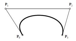
Figure (1): Simple Cubic Bezier curve polygon with its control points. [6]
