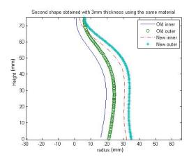
Figure (10): The second shape of the candle holder after changing the volume.
