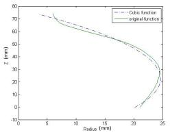
Figure (5): Cubic Bezier Curve vs. the original curve.
