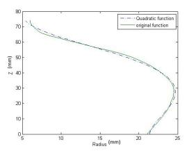
Figure (6): Quartic Bezier Curve vs. the original curve.
