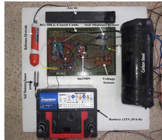
Figure 2: The built ICCP system components.
