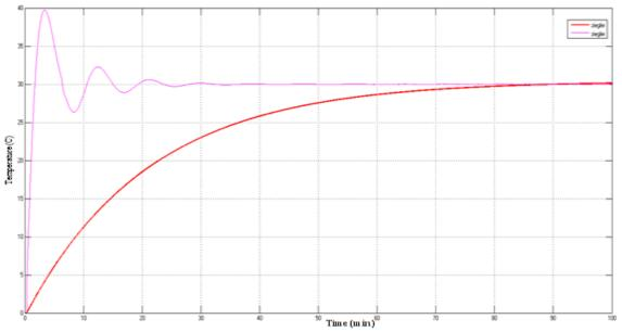
Figure 9: Response of temperature at 50% step on feed flow rate.
