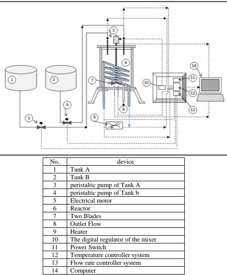
Figure 1: Schematic diagram of laboratory CSTR reactor system
