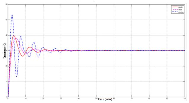
**Figure 4:** Comparison among Temperatures (°C) of CSTR for three Methods at 50% step change on water flow rate in coil vs. time (min)
