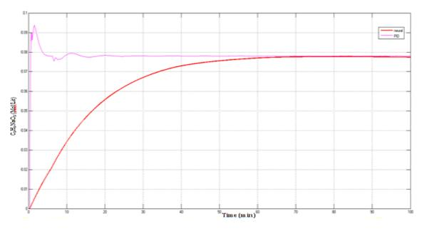
Figure 10: Response of product at 50% step on water flow rate in coil.
