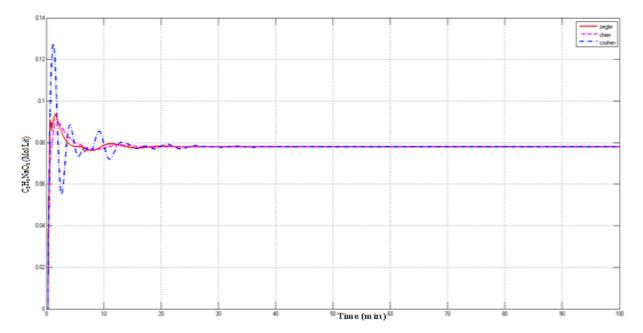
Figure 3: Comparison between Concentrations (Mol. /Lit) of sodium acetate for three Methods at 50% step change on ethyl acetate flow rate
