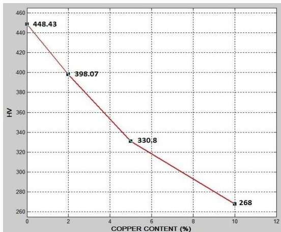
Figure 8: Vickers micro hardness as a function of copper content for compacting pressure 450MPa.
