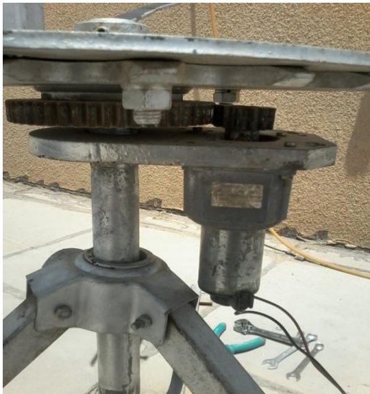
Figure 3a: DC gear box
