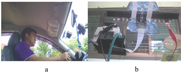
Figure 6. Experimental setup of (a) driver position and (b) IR camera setting where IR LEDs, IR camera, and Raspberry Pi are shown in red, yellow, and blue rectangle boxes, respectively.
