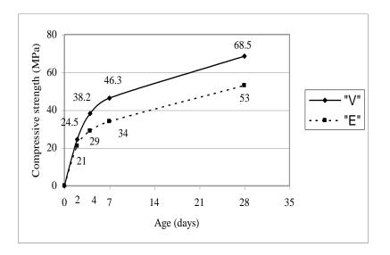
Figure 4. Compressive strength growth in time
