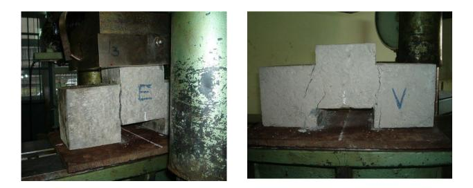
Figure 7. Shear strength test
