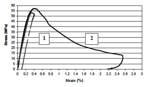
Figure 8. Stress-strain diagrams of both series of concrete, 1- reference and 2 – FRC
