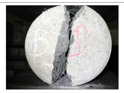
Figure 6. Spliting tensile test - Steel fibers continue to bridge the crack after the breakage of the specimen
