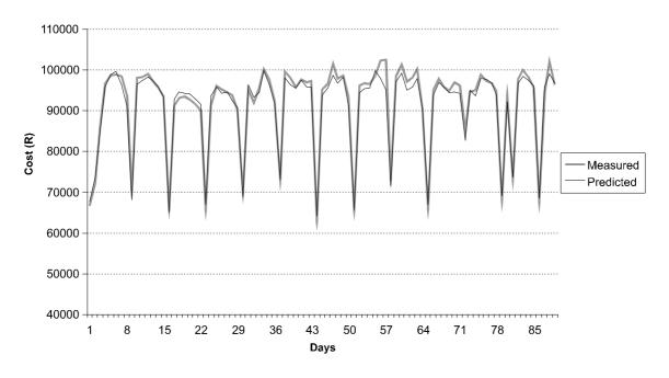
Figure 5: Load prediction model verification at Kopanang
