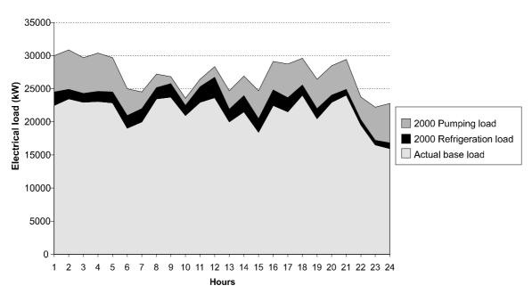
Figure 4: The composition of the predicted total load profile at Kopanang
