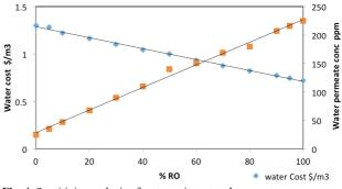
Fig. 4. Sensitivity analysis of water unit cost and permeate concentration
