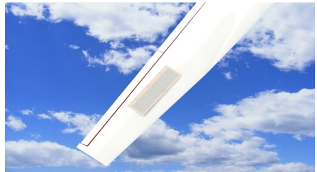
Fig. 25. Photography performed by SolidWorks program in a full scale representing the wing UAV with P-ESPAR antenna placed.
