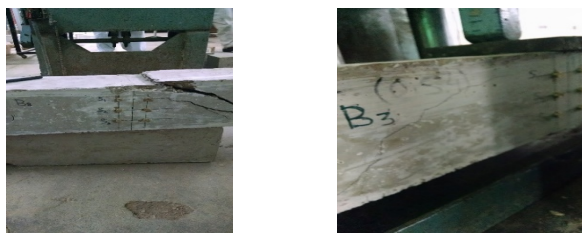
Fig. 5. Failure of beams
