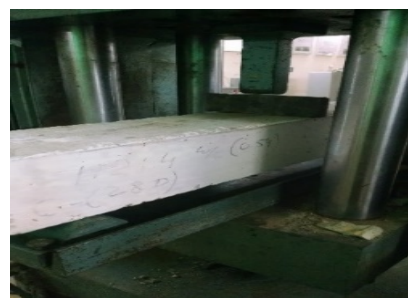
Fig. 3. Beam under central point load
