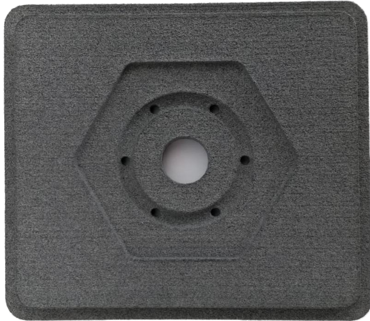
PA12 surface after manufacturing
