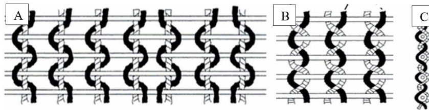
Fig.1: Plain leno weaving structures: warp yarns white barred: stationary black: crossed, Plain white: weft [1], [3] A: one-twist two gauze B: two-weft gauze C: Crosscut view of leno fabrics.
