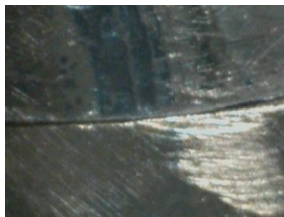
Figure 11: Image of the distal abutment-framework interface gap (100 \times magnification)
