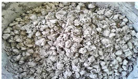
Fig. 8. Concrete sample mix with 16% rubber crumb
