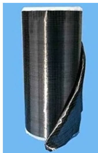
Fig. 3. Carbon FRP sheet for external structural reinforcement (photo from http://www.fortecstabilization.com )
